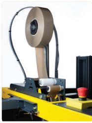
Possibility to order the version for K12 head for 75 mm tape width, in this case the minimum box width has to be 170 mm.
