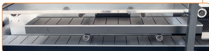
Dedicated Drying Sections for each station
