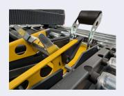
With few operations it is possible to easily change the cutting system to set different tape legs (from 30 to 70 mm), securing the box according to the needs.
