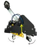
A special configuration allows to pneumatically control both cutting system and adhesion rollers, avoiding impact and tape application on boxes/packs that don't require to be sealed (ByPass function)
