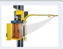
The machine can wrap loads either manually-allowing occasional, operator-controlled wrapping—or automatically, with selectable programs for single or double wrapping, with or without a top sheet, based on the load type.
