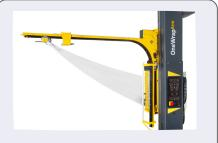
OneWrap Arm automatically attaches and cuts the film at the beginning and end of the wrapping cycle, eliminating the need for any manual film handling. This significantly improves operator ergonomics, reduces repetitive strain, and speeds up the wrapping process.
