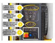
The operator selects the bestsuited option for the load and saves all wrapping parameters speed, tension, rotations, and delays. Up to 9 + I custom programs can be stored and recalled by number for quick, consistent wrapping.
