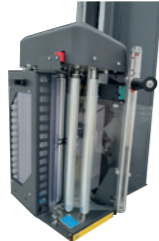
Roping System available for Viking PW and DM, pneumatic device that shrinks the film to create a rope: it gives stability and strength to the filming
